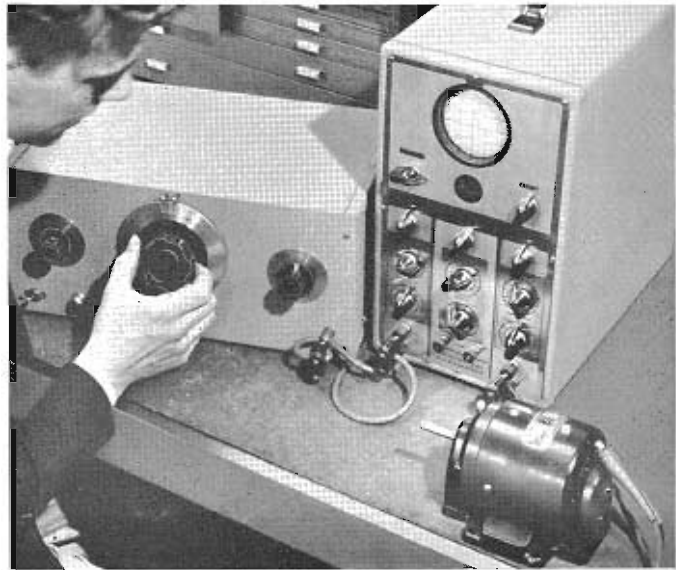
Frequency of the output voltage of a dynamotor is being measured with a Model 200B.
