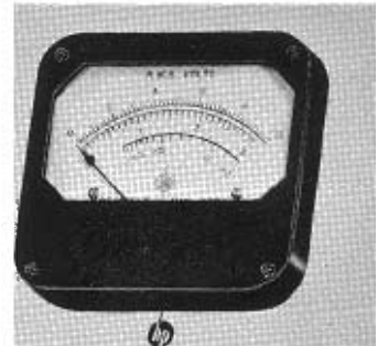
Meter face on 400A. Note both voltage and D. B. calibrations.
