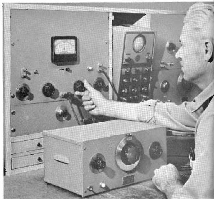
The 325B Distortion Analyzer is being used to measure the total harmonic distortion of a Model 200B on the production test bench.
